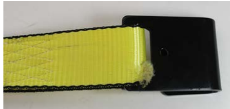
Figure 8 Tear in Webbing at the Fitting.
